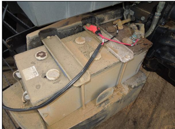
Example battery connection: MXM / TM series tractors
