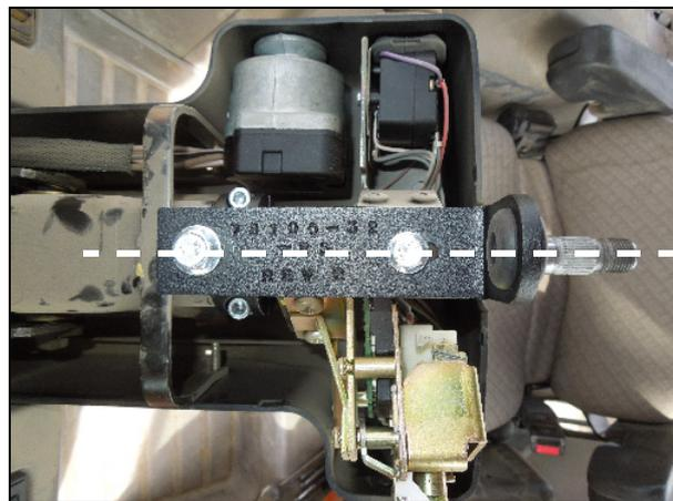
Bottom bolt aligned on centerline
