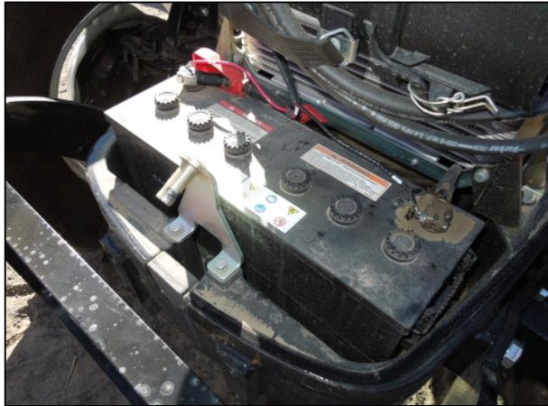
Example battery connection: T50x0 / Farmall U series tractors
