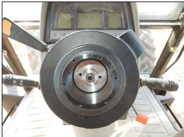
Align the spline teeth of the steering shaft and lower adapter by hand.
